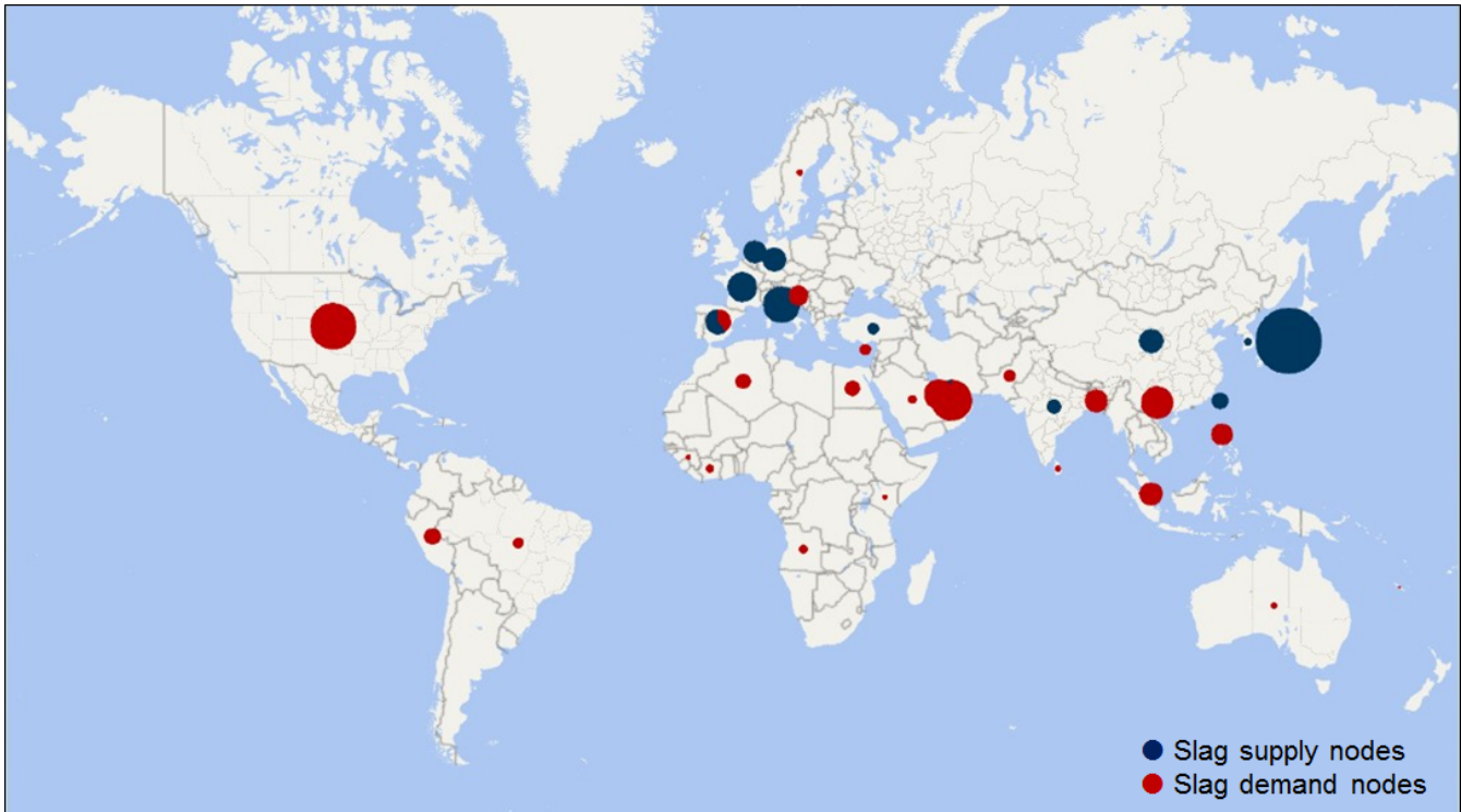
Figure 1 – Slag supply chain network
