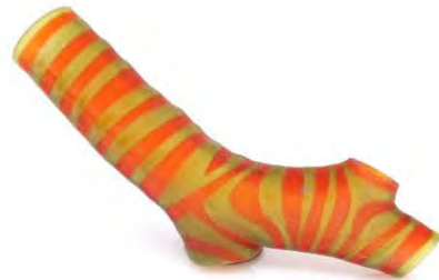
Multi-material Bronchial Tube Model Elastomer (green), Rigid (red)
